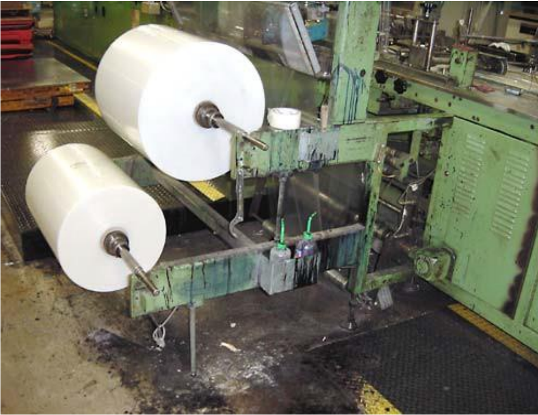
Original SITMA film unwind reel stand. Unwind is NOT powered, resulting in film stretch and inaccurate registration when using printed film.
