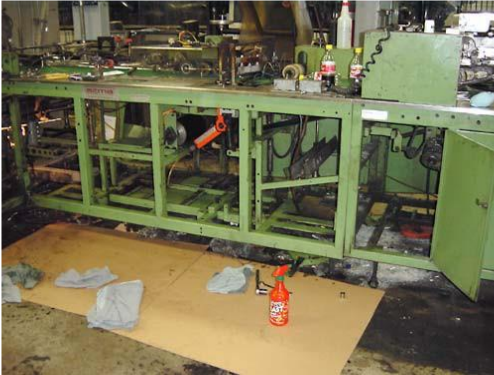
The C80/750 wrapper frame is completely “cleaned-out during the re- manufacture process
